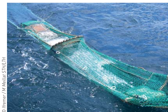
Deploying the combination of three selective devices: Nephrops grid, cylinder and square-mesh net panel (trawl belly) for Nephrops
