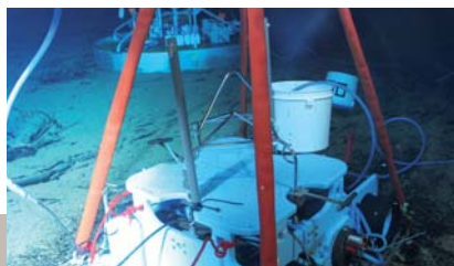
The geophysical node was moored in the centre of the lava lake which is characteristic of the Lucky Strike hydrothermal field for observations
